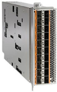
Figure 8. 20-Port 10-Gbps Unified Port Line-Card Expansion Module
